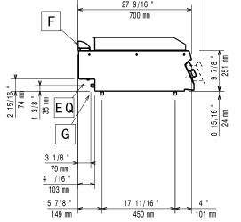
EQ = Equipotential screwG = Gas connection
